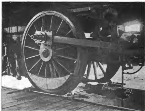
Fig. 5021. Farrington's Valve Setting Machine, Fitted with Mills Power Attachment. Sherburne & Co.
